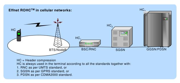
Effnet ROHC<sup>TM</sup> is highly portable, platform and endianness independent, software. It's modular design is configurable at compile and run time. This makes it suitable in various environments including multi-thread, multi-core, memory and system challenged etc. Effnet ROHC<sup>TM</sup> focuses on standards compliance and efficiency, compression, system as well as operational level.
