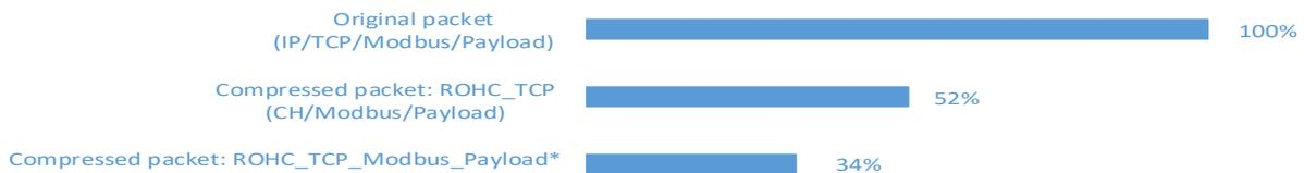
Figure 4. Packet size is significantly reduced after the application of header & payload compression
